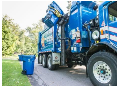
Figure 19. Automated Side Load Collection. Provides a cleaner, safer, more efficient residential collection.
