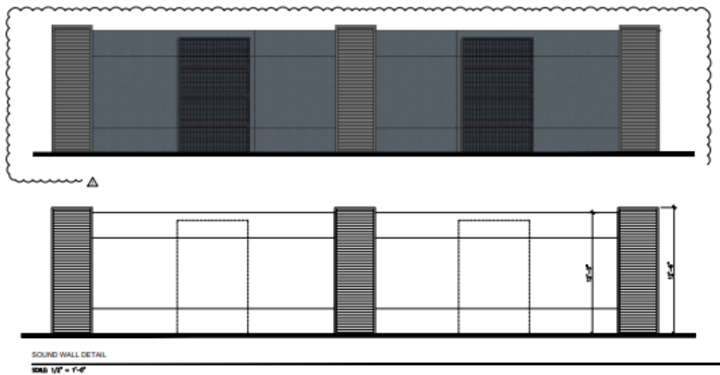
Figure 7: Loading Dock Screen Wall Detail
