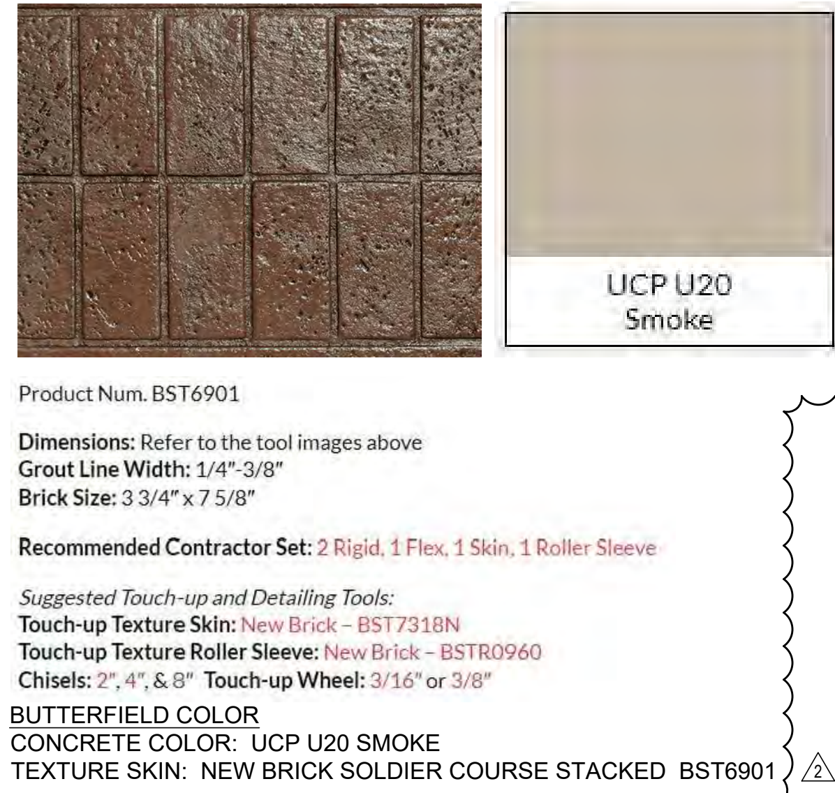
STAMPED CONCRETE DETAIL SCALE: NO SCALE
