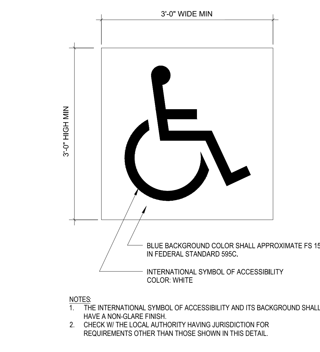
ACCESSIBLE SYMBOL AT ACCESSIBLE PARKING STALLS SCALE: 1" = 1'-0"
