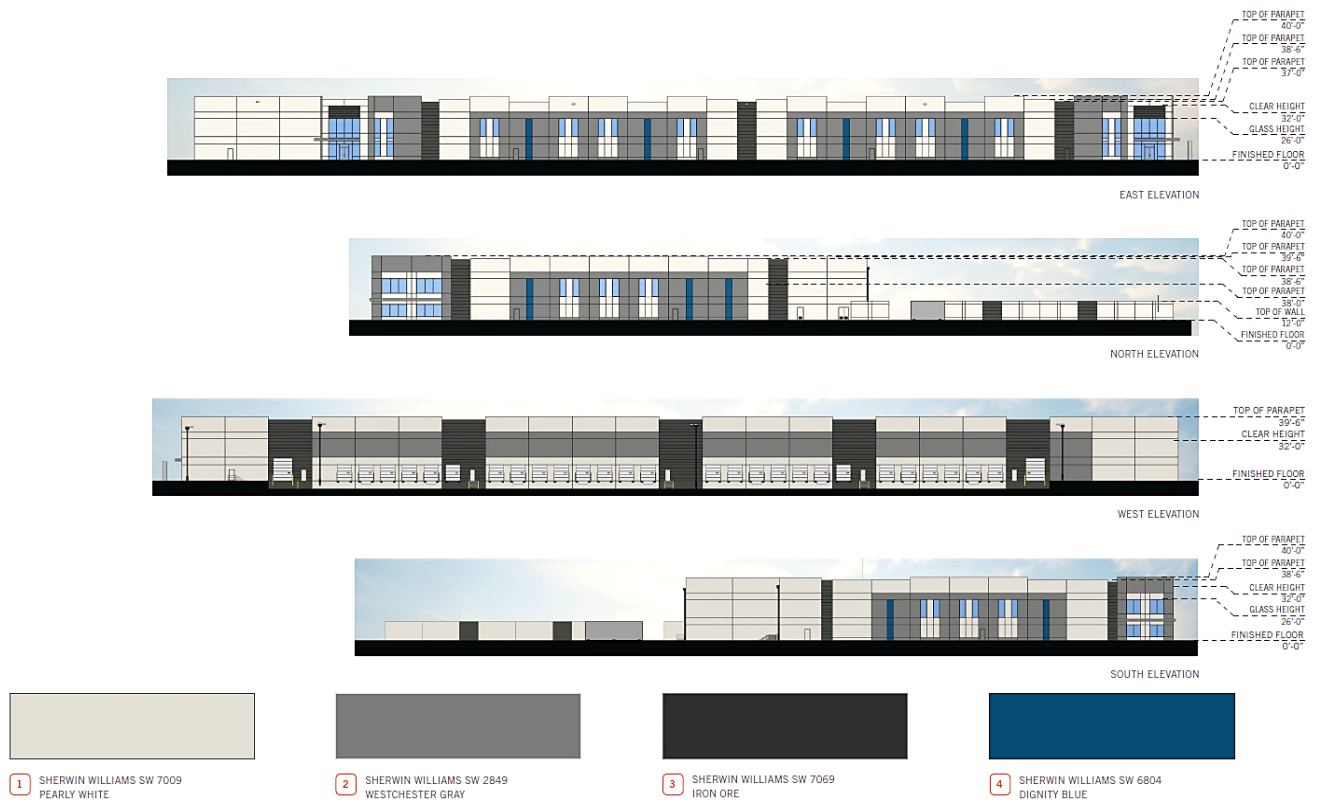
Figure 3: Propose Building Elevations
