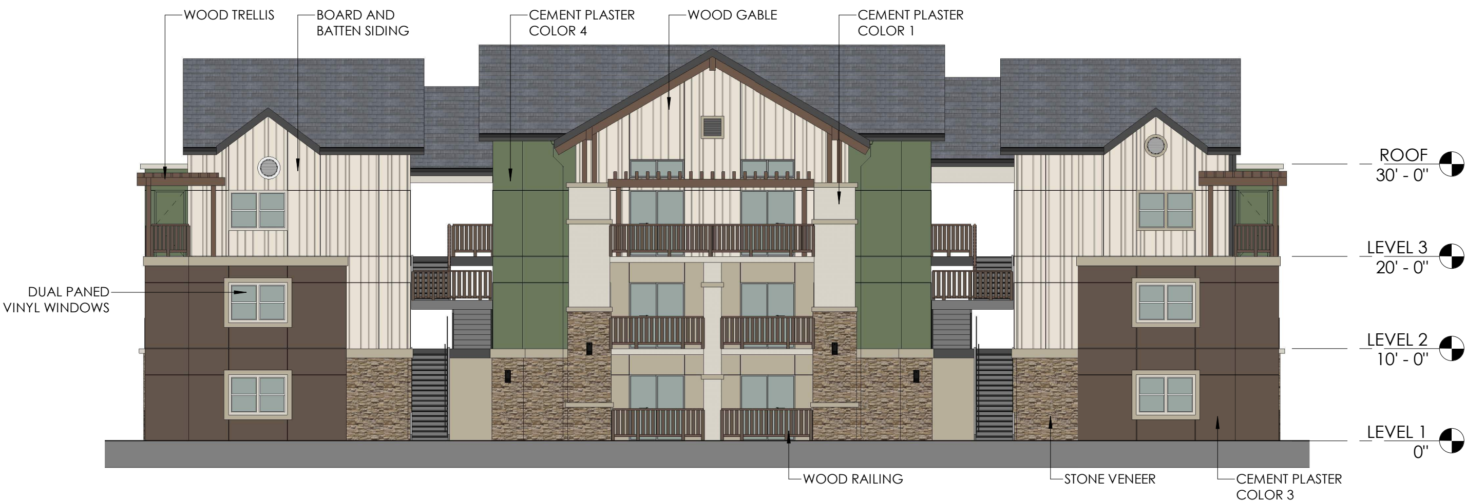
BLDG D - ELEVATION 4 3/32" = 1'-0"
