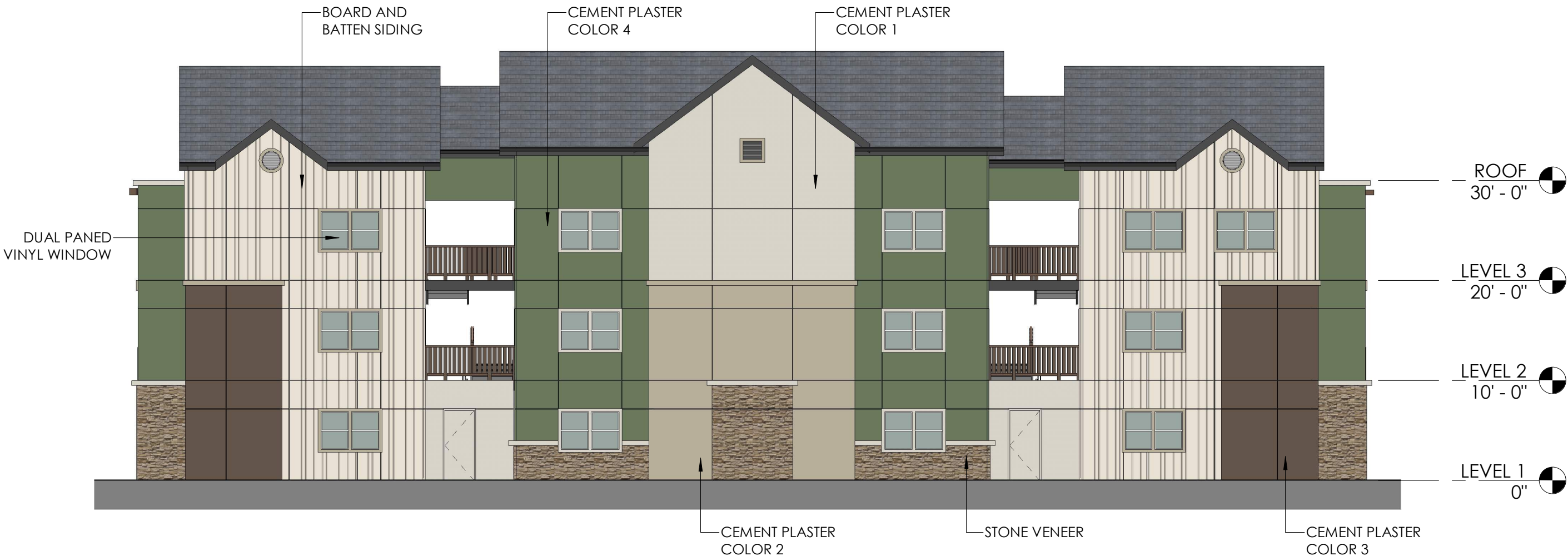
BLDG D - ELEVATION 5 3/32" = 1'-0"
