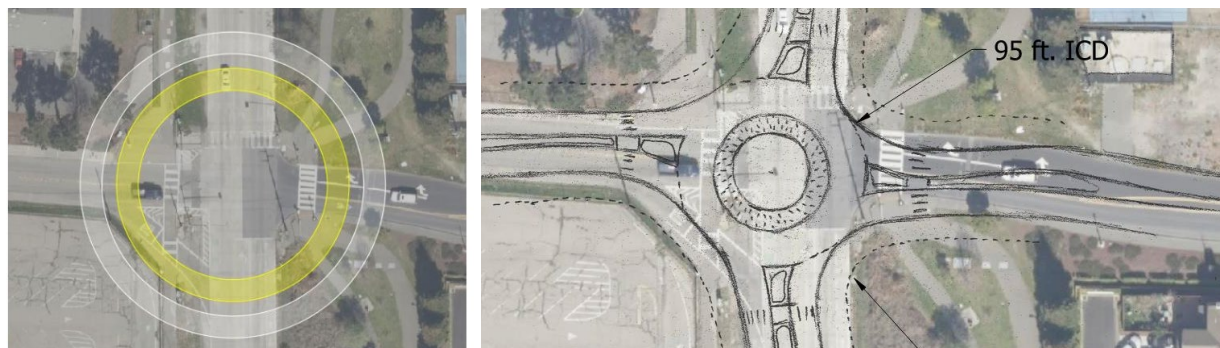
Figure 4: Roundabout Footprint Estimate Leading to Viable Concept.
