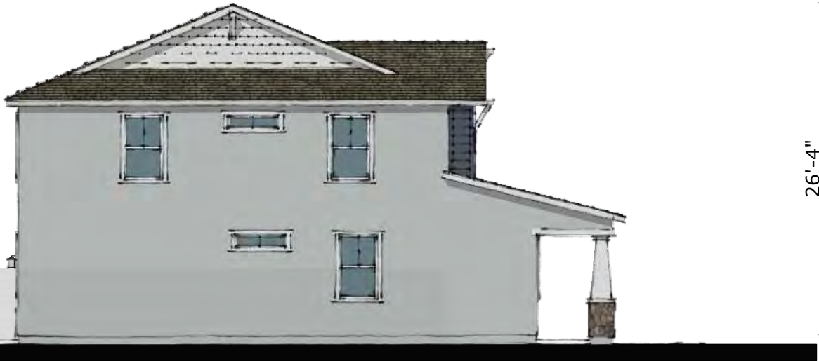
LEFT ELEVATION SCALE: 3/32" = 1'-0"
