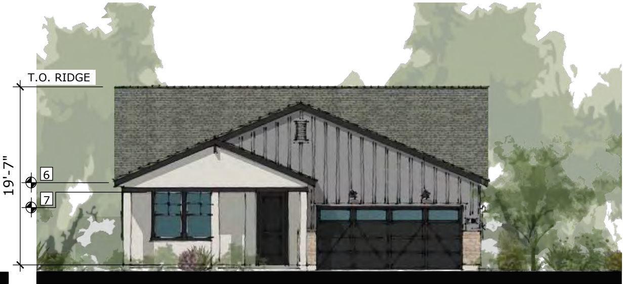
FRONT ELEVATION SCALE: 3/32" = 1'-0"
