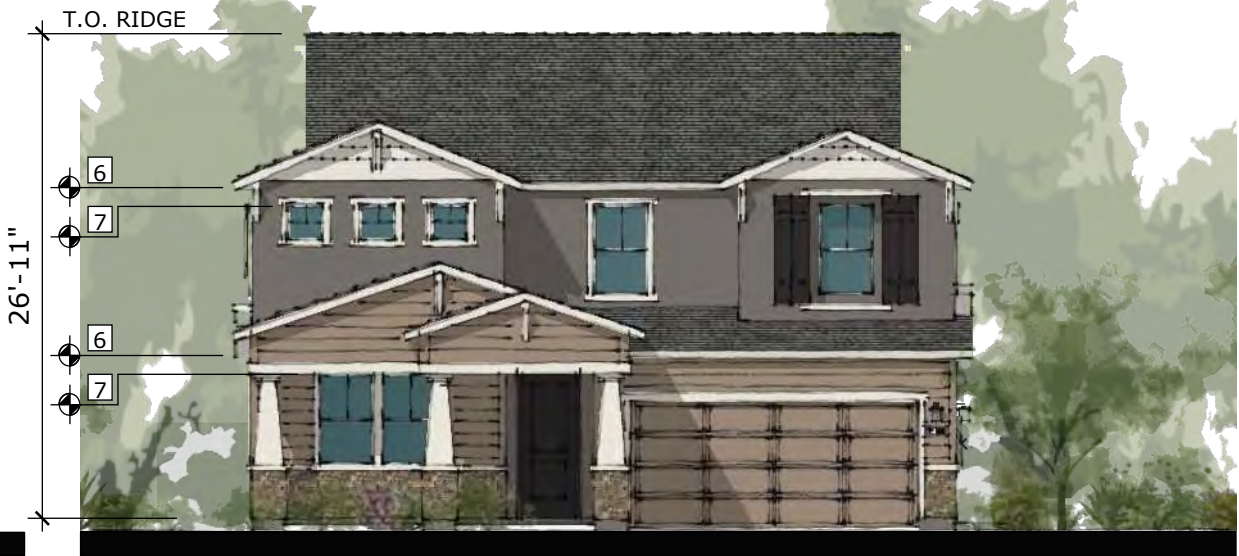
FRONT ELEVATION SCALE: 3/32" = 1'-0"
