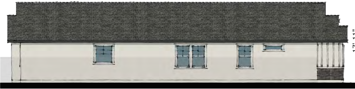
LEFT ELEVATION SCALE: 3/32" = 1'-0"
