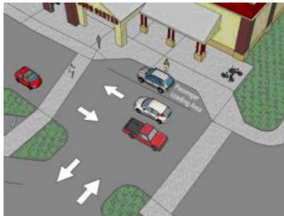
Figure 23.719-7: Passenger Loading Areas
