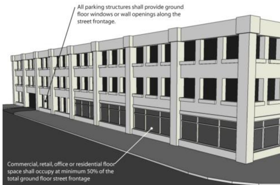
Figure 23.719-3: Parking Structure Design Requirements
