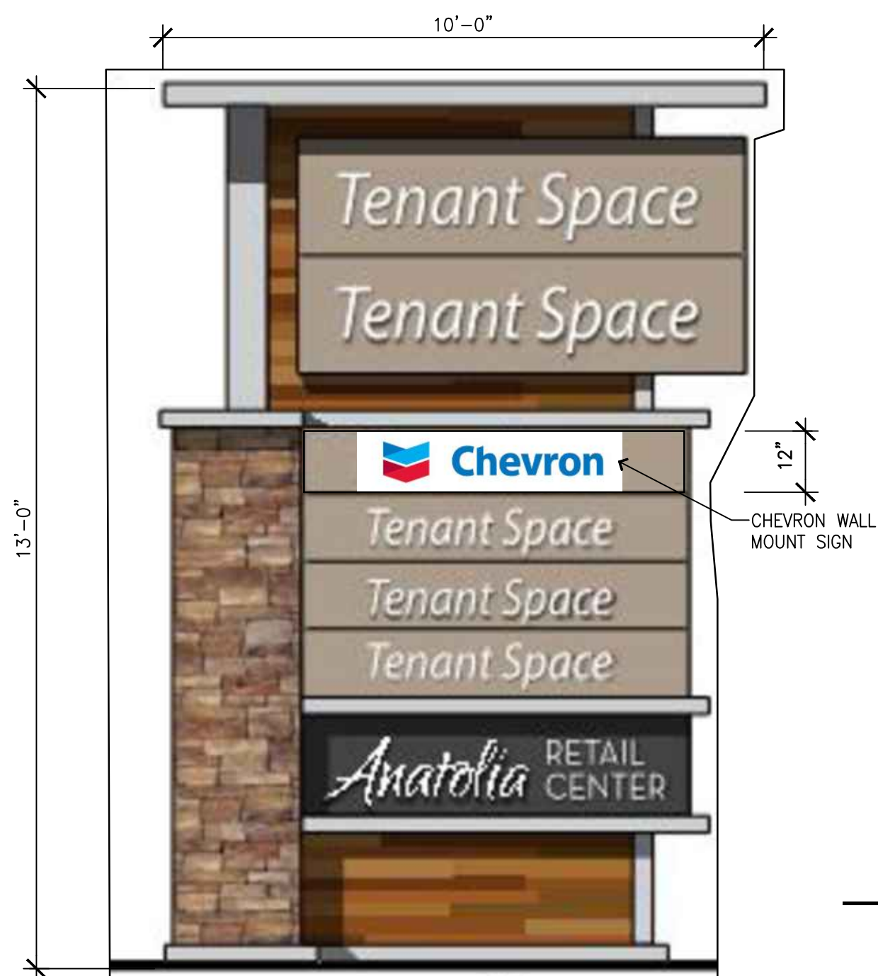
N MULT-TENANT PYLON SIGN SCALE: 1/2" = 1'-0"
