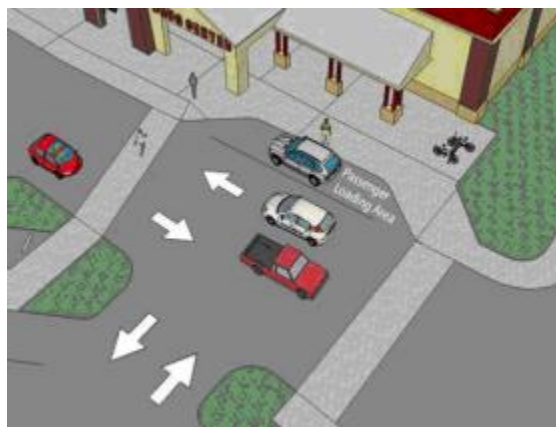
Figure 23.719-7: Passenger Loading Areas
