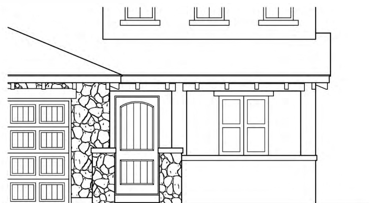
PARTIAL FRONT ELEVATION AT OPT. COURTYARD WALL
