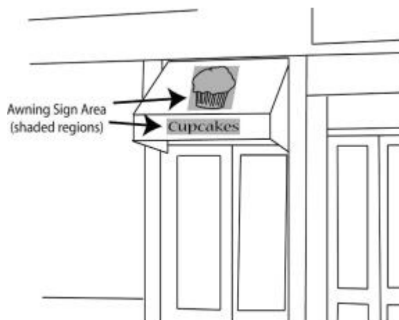
Figure 23.743-6: Awning or Canopy Sign Area
