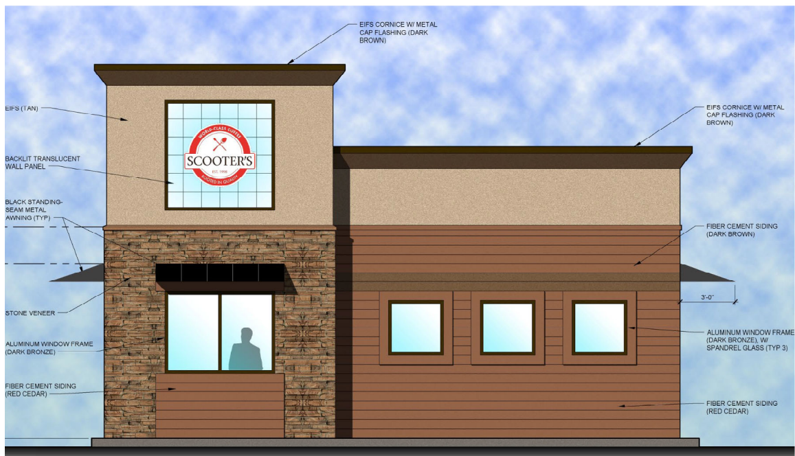
FIGURE 3 – STREET FACING ELEVATION
