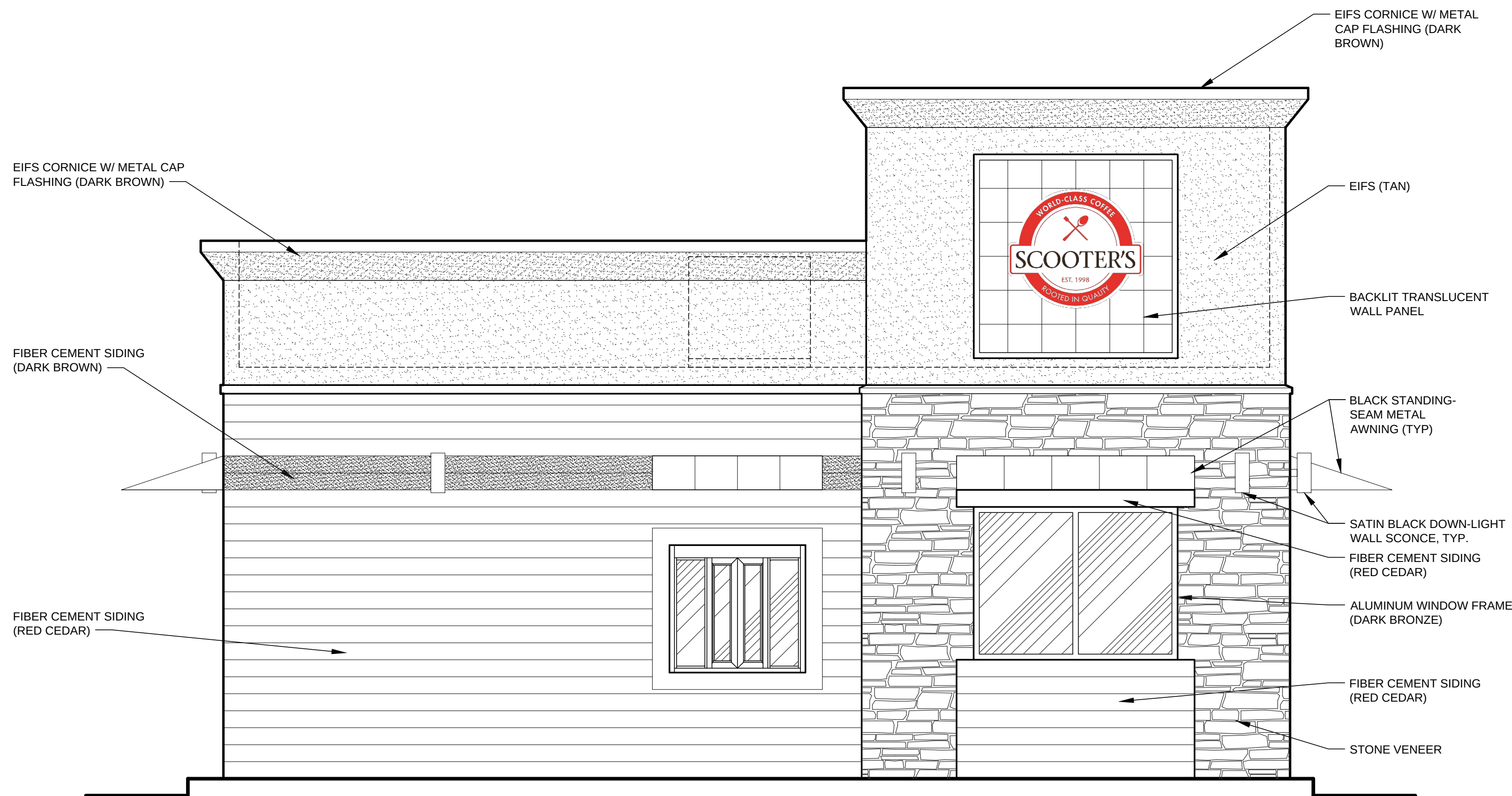
A1 EXTERIOR ELEVATION (SOUTH) SCALE: 3/8" = 1'-0"
