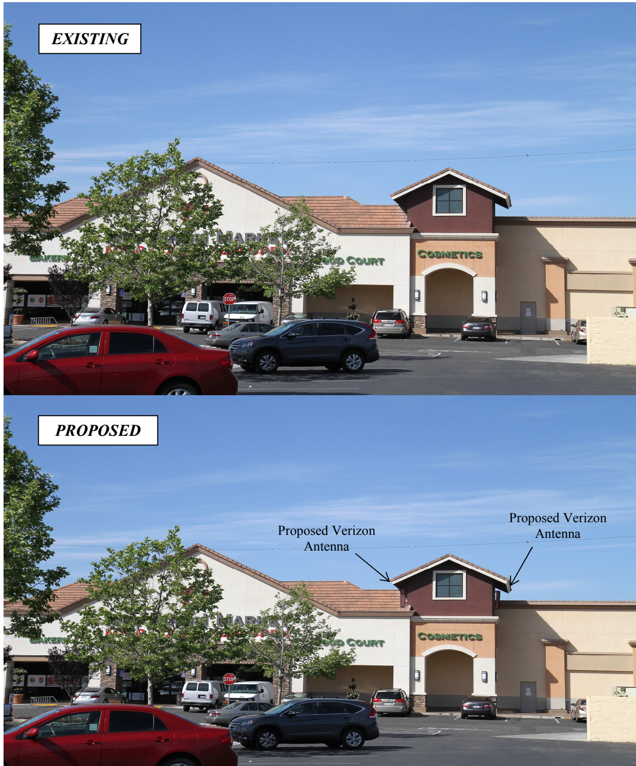
Figure 2: Building Elevations Existing & Proposed
