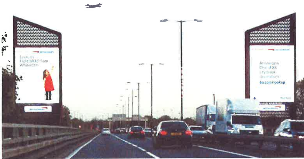
Figure 3. A pair of digital billboards spanning a 4-lane highway in London. The signs are used together to display parts of a message that encourage the driver to look at both signs sequentially.
