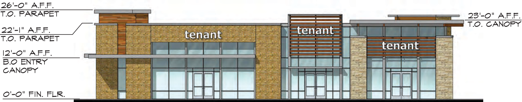
S2 Building | Front Elevation Scale 1/16"=1'-0"
