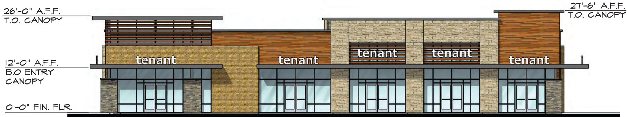
S1 Building | Front Elevation Scale 1/16"=1'-0"
