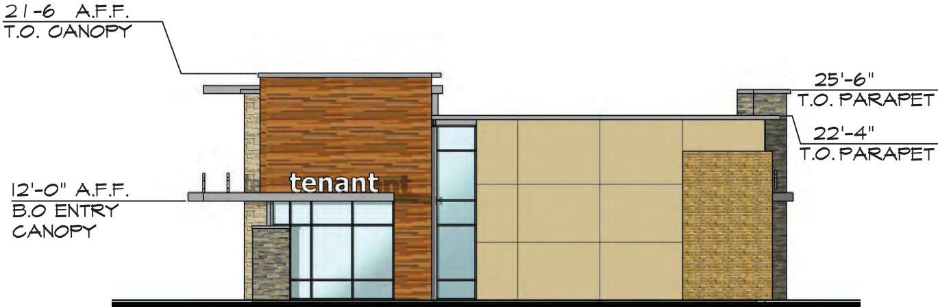
S1 Building | Right Elevation Scale 1/16"=1'-0"
