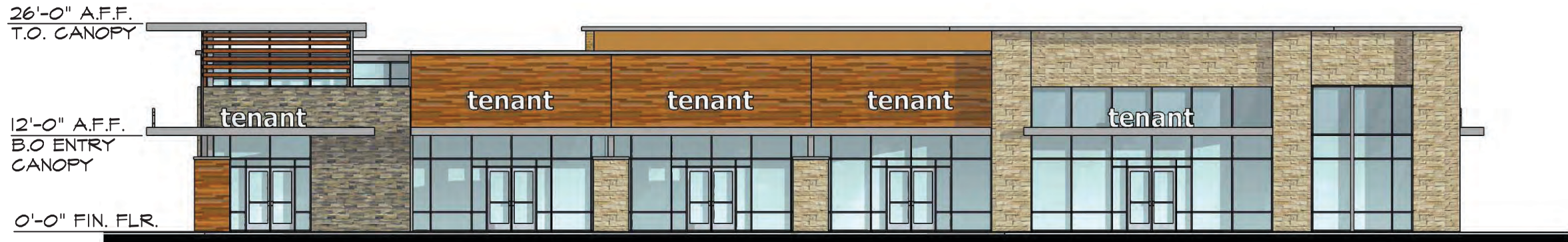
S6 Building | Front Elevation Scale 1/16"=1'-0"
