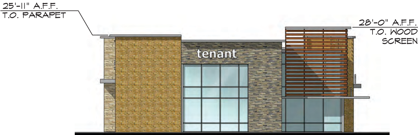
S5 Building | Left Elevation Scale 1/16"=1'-0"
