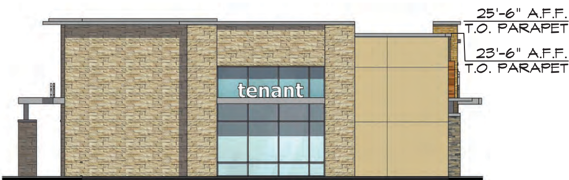
S6 Building | Right Elevation Scale 1/16"=1'-0"
