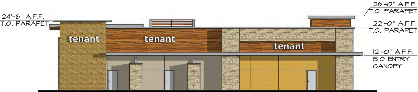
S2 Building | Rear Elevation Scale 1/16"=1'-0"
