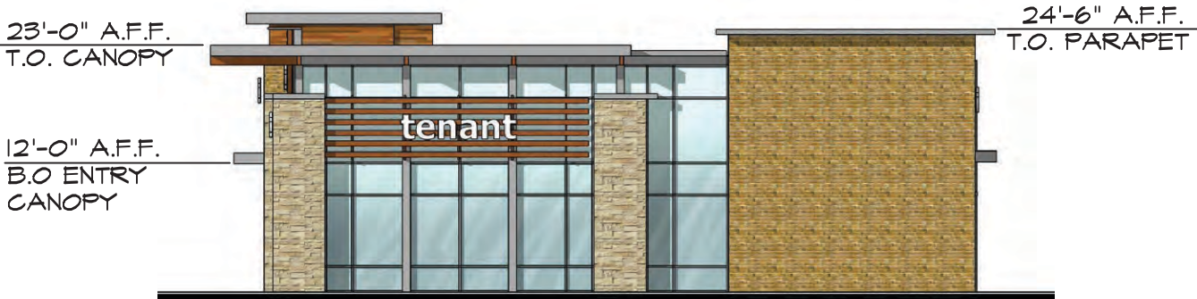
S2 Building | Right Elevation Scale 1/16"=1'-0"
