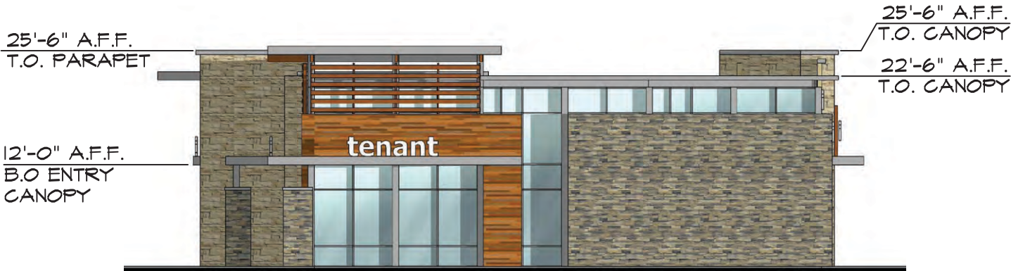
S3 Building | Right Elevation Scale 1/16"=1'-0"
