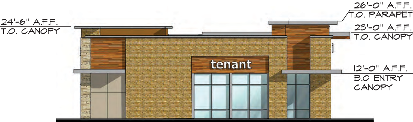
S2 Building | Left Elevation Scale 1/16"=1'-0"
