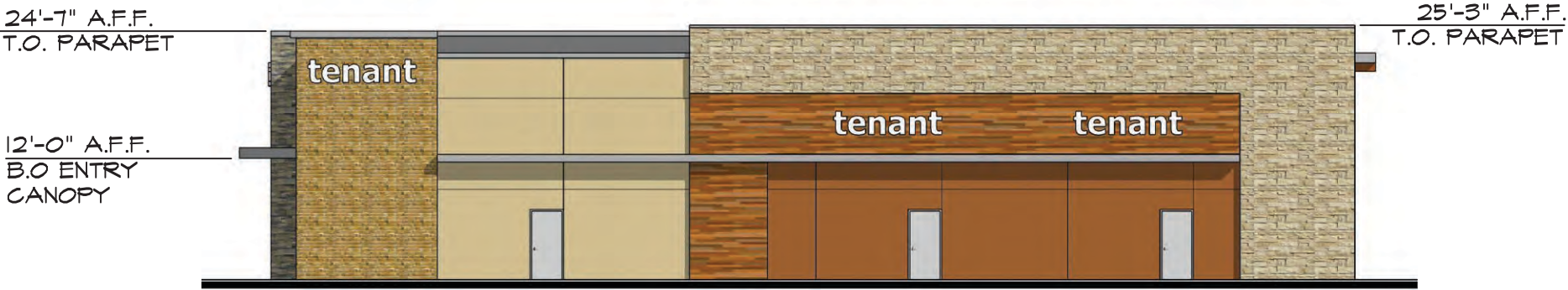
S4 Building | Rear Elevation Scale 1/16"=1'-0"
