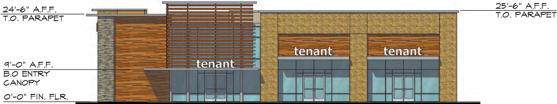
S5 Building | Front Elevation Scale 1/16"=1'-0"
