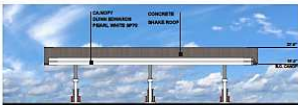
GAS CANOPY-TYPICAL SIDE ELEVATION
