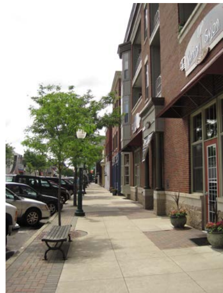
Nonresidential local street with tree wells and lighting placed in the landscape strip
