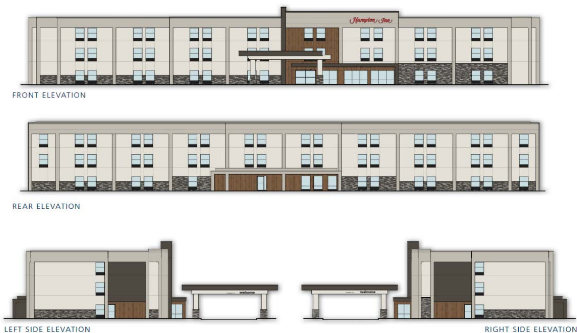
Figure 3: Proposed Façade Renovation Elevations
