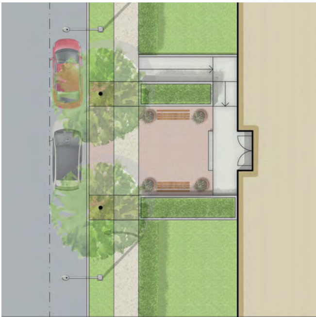
Parking 8'-0" 5'-0" 5'-0" 20'-0" 20'-0" Typical Setback 5'-0" Minimum Sidewalk & Landscaping 4'- 5' Planting Strip
