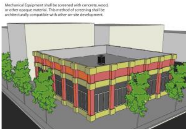
Figure 23.731-3 4: Screening of Roof-Mounted Equipment
