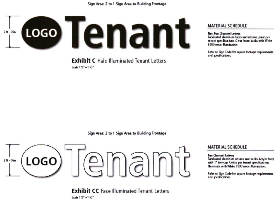
Figure 5.3 – Wall/Fascia Signs Example
