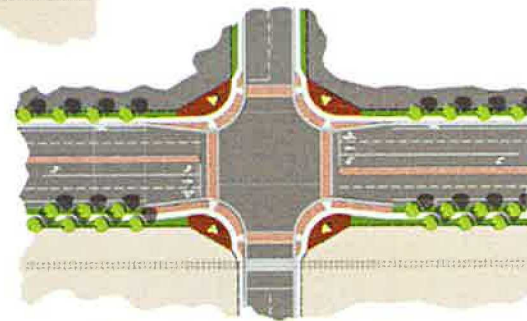
INTERSECTION WITH BULB-OUT FEATURE
